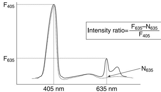
**Fig. 1** Spectrum of protoporphyrin IX-fluorescent tissue demonstrating the peak at 635 nm. The fluorescence intensity ratio was calculated as the ratio of the peak emission intensity to reflected excitation light intensity after subtracting the extrapolated autofluorescence curve.  $F_{405}$  and  $F_{635}$  indicate the absolute values of the fluorescence intensity at 405 nm and 635 nm, respectively;  $N_{635}$ , the autofluorescence at 635 nm.
